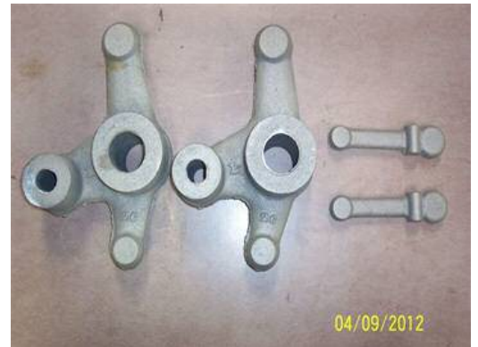
Casting for two steam arms and trip levers. Holes through the steam arm castings were formed by cores. Core prints on the pattern locate the cores in the sand mold.
