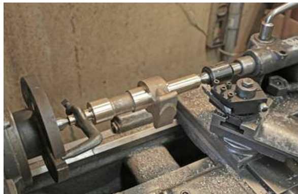
Left: The finished trip shaft pattern with two brass castings Right: Casting being turned on the lathe
