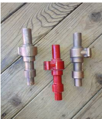
Left: The finished trip shaft pattern with two brass castings Right: Casting being turned on the lathe
