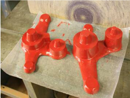
Finished steam arm pattern. The pattern is split at the parting line to make molding easier.
