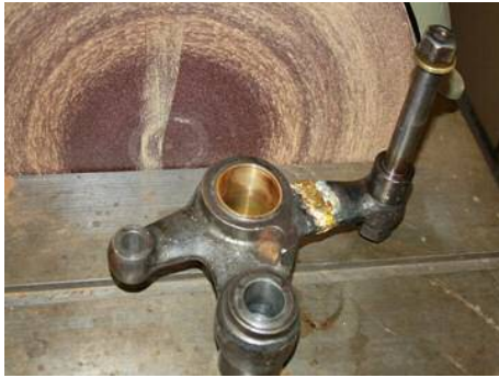
Steam arm for the Corliss engine showing brazed repair
