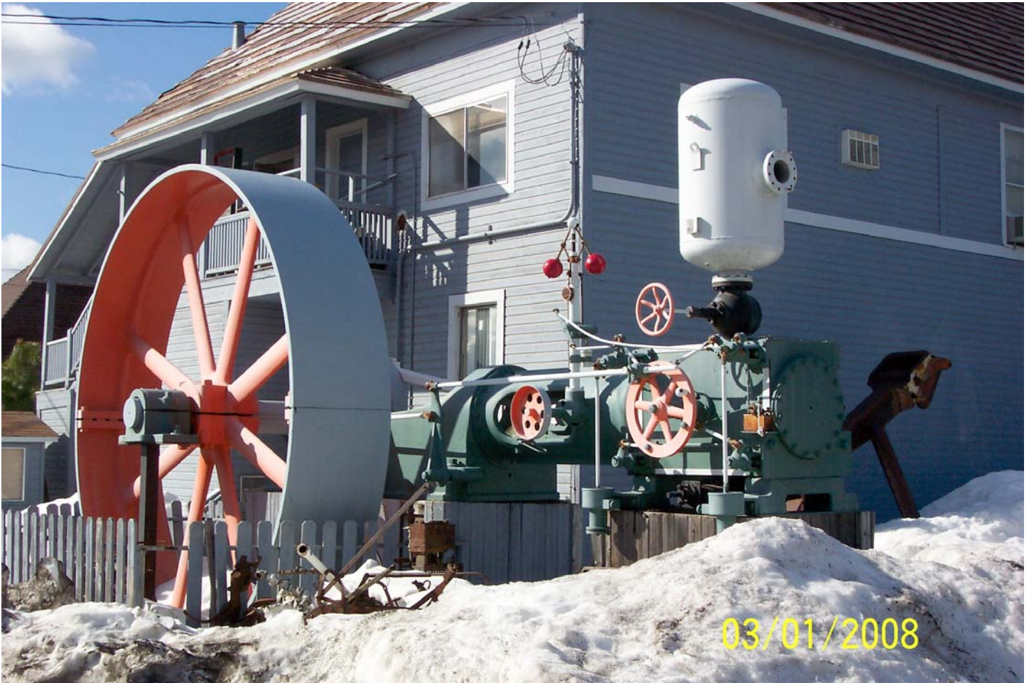
1903 Allis Chalmers Corliss Steam Engine Powered the McCloud Lumber Co. Sawmill 1903 - 1979 McCloud, CA
